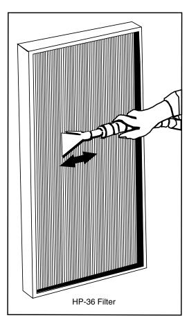
**Note:** Occasionally, remove the filter and high-pressure wash (10" away) only the pleated filters to remove trapped particulate.
