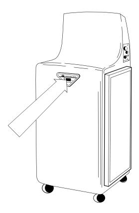
The digital read-out on the front of the machine indicates the airflow volume in cubic feet per minute (CFM). When the machine is first started the reading should be at least 1000 for the Duster 1000, and 2000 for the Duster 2000 in the high position of variable speed control.
